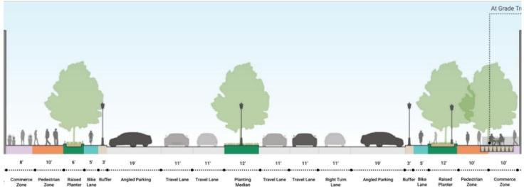
For reference: 5 ft bike lane is a minimum and requires one-way, single file traffic. Cars and trucks that overhang the buffer from curb to sidewalk will effectively reduce the buffer.
